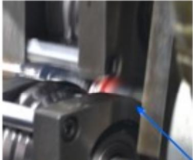
Hot rolling to form required shapes with controlled thickness and hardness
